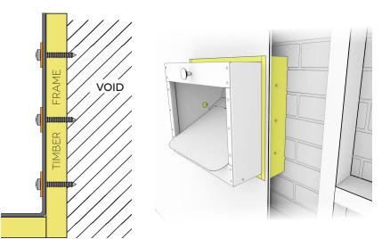
Chutes mounted in wall types such as **Brick Veneer** or similar styles that have hollow sections between the outer and inner wall, will use the **I4G x 32mm** timber screws and mount directly to the timber frame installed by the contractor when cutting and cladding the book chute hole.
