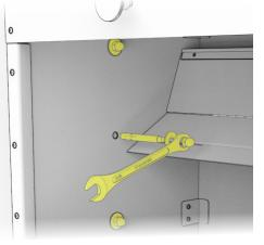
Mounting through timber frame into masonry:(6) DYNABOLT D I 0075 :98002(6) 23mm OD Flat Washer :85429(6) M8 Dome Nut Chrome :98003
