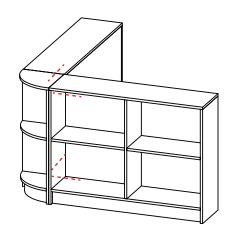
In the Top & Bottom rear coreners of each unit, drill a small 5mm hole through both adjacent units and fasten together with the provided bolts
