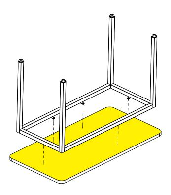
Place table top upside down on a flat surface. Center frame on the bottom of the table top and measure 50mm on each side.
