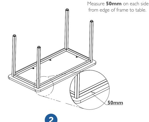
Locate the D-tab holes and screw the frame into the table top using a drill. Proceed to flip the table upright.
