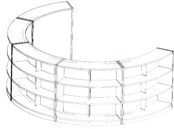
In the Top & Bottom corners of each unit, drill a 5mm Dia hole through both units and fasten together with the provided bolts
